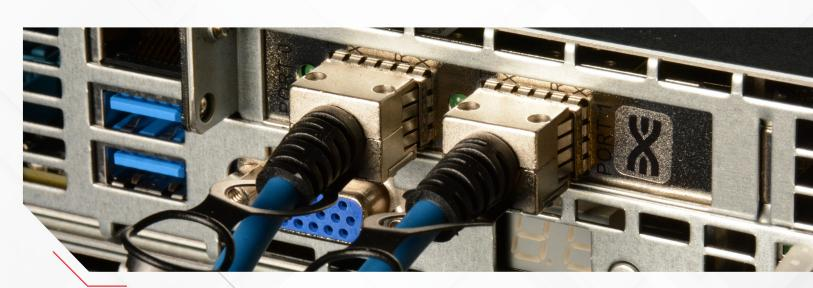
High speed interconnect assemblies can offer a significantly lower upfront cost over transceivers and jumper cables.
