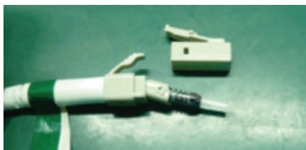
Connector break after 19.4N for 60 seconds at 90° degree pull
