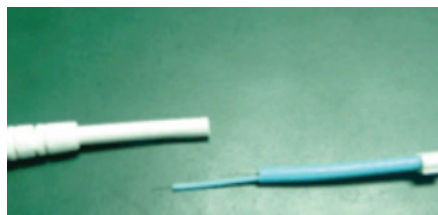
Fiber break after 50N axial pull for 60 seconds
