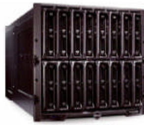
Blade Chassis Servers
