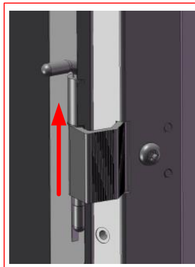
DOOR HINGE PIN (Slide up and out)
