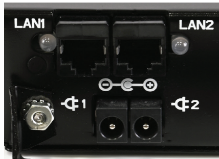
REDUNDANT POWER & ETHERNET
