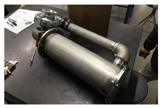
As one can see, the compressor outlet (shown on top left of the last picture) was connected to the inlet pipe via metal zip ties over a silicone coupler designed to withstand high temperatures. This design was chosen mainly because there are no other alternatives to join the two parts together, added by the facts that:
