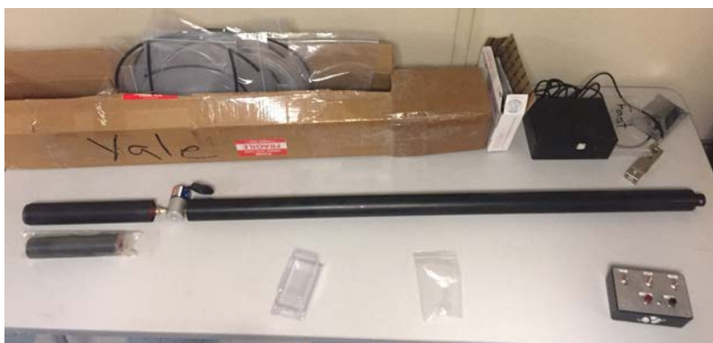
Fully machined combustion chamber, preliminary valve assembly, and oxidizer tank alongside ground support equipment prototypes with nitrous fill tubing in the box above
