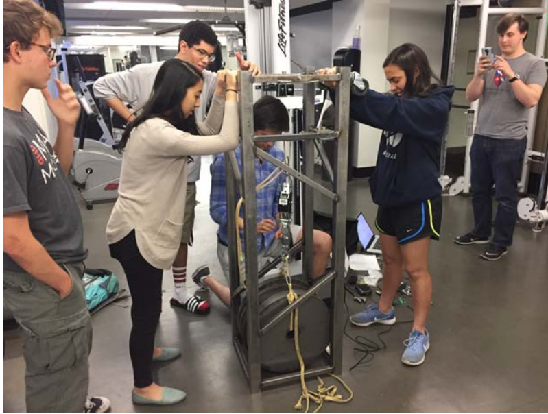
Team members performing medium-level stress testing of load cell mounting system
