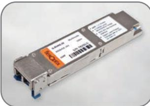
The quad small form factor pluggable (QSFP) is a compact, pluggable transceiver. QSFP+ transceivers support 40G Ethernet, 20G/40G Infiniband and other communications standards. QSFP+ modules increase port density by a factor of 4 times when compared to SFP transceivers.
