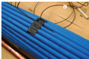
Photo 2. Placement of temperature sensing Thermocouple
