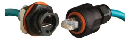
Siemon's industrial solution achieves an IP 67 rating primarily by means of a sealed RJ-45 plug and outlet. The plug's body has a unique bayonet-style-coupling
