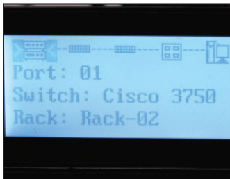
A complete circuit trace can be viewed on-screen at the MCP or DCP
