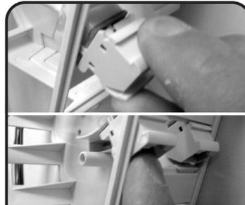
**5a** For MAX modules, align the top of jack with outlet opening... and angle down until it snaps into place. Note: Snap icon into module prior to snapping module into MX-MMO.
