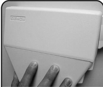
**9** Align the housing cover over the base and insert the top latches of the cover into the slots located in the upper wall of the base. Rotate the cover into position until the bottom latches snap into place.
