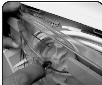
**7** Align the tray into position and push the center latch down to lock the tray to the base. Be careful not to pinch fibers.
