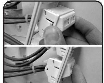
**5b** Insert CT couplers into the appropriate opening and push until it snaps into place.
