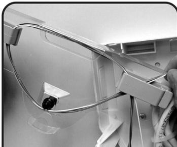
**6** Store excess fiber using fiber tray to make sure proper bend radius is maintained.
