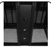
Place the VPC over the (4) shoulder bolts and hook the back plate into place.
