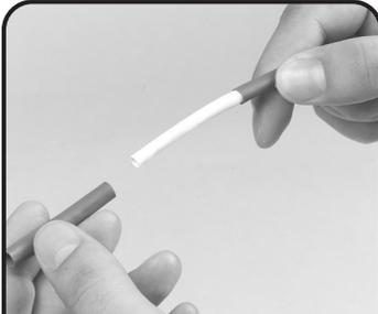
**3** After removing the sheathing, the inner jacket will be visible.
