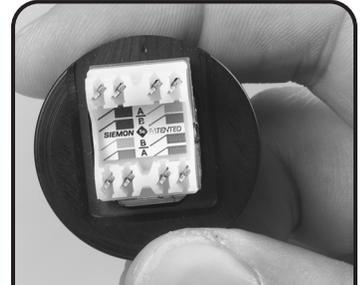
**6** View the color code label on the outlet to determine the proper location of conductors based on preferred wiring scheme.
