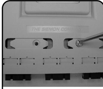
**13** If desired, use the last two self-tap screws to secure the cover to the base as shown.
