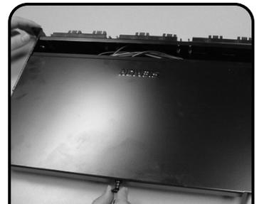
**10** Install top cover by pushing onto enclosure tabs and then sliding forward under over-hang at front. Engage the push-pull latch to secure. Mount enclosure onto rack using hardware provided.
