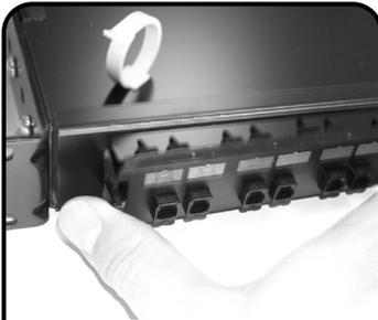
**3** Align the adapter plate latches with the respective cutouts in the mounting plate and push the adapter plate inward until it snaps into place.
