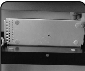
**7** If optional splice tray is used, install using four velcro style tabs as shown.
