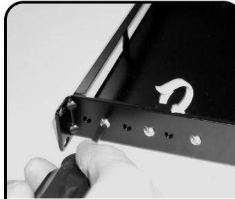
**1** Tray can be mounted to a rack in a protruding, flush or recessed position. Once determined, secure the mounting brackets to each side of the enclosure using the two screws provided.
