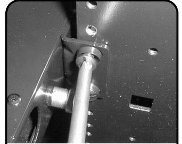
**2** Mount enclosure onto rack using the four screws and plastic washers provided.
