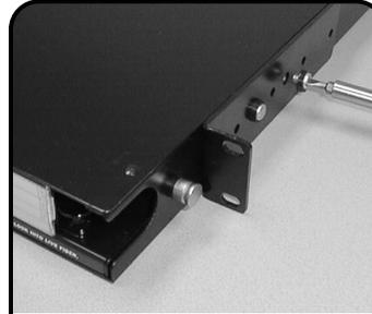
**1** The enclosure can be mounted so that the protrusion from the front of the rack is either 51mm (2 in.) or 102mm (4 in.). Align the mounting bracket holes with the appropriate holes in the enclosure and secure a mounting bracket to each side of the enclosure using the two screws and plastic washers provided.
