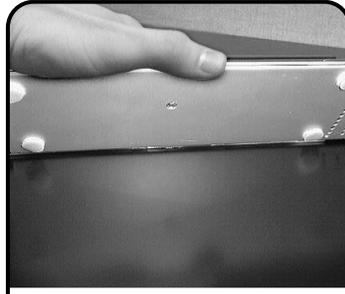
**13** If optional splice tray is used install using four velcro-style tabs as shown.
