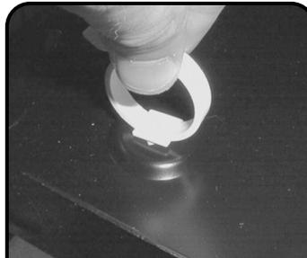
**8** Install four fiber management clips in the rear of the enclosure by inserting into appropriate holes and turning 45 degrees to lock into place (clip opening should face the outer walls of the enclosure).
