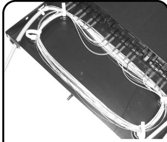
**12** Once cable is secured, terminate fiber per manufacturer's specifications and route cable slack through fiber management clips. Mate connectors to appropriate adapter and slide tray to the closed position by disengaging the rear latch head.
