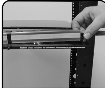
**4** Once tray is out, remove the label bracket by disengaging snap latches on left and right side of holder.
