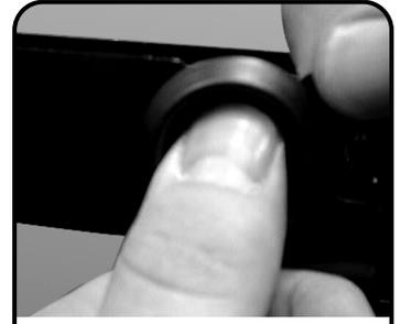
**14** For dust proofing - Install feed-through grommet into un-used access hole as shown.
