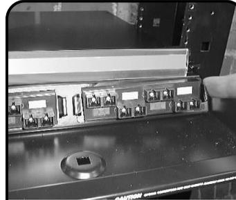
**5** Align flat Quick-Pack latches with the respective cutouts, in the adapter plate bracket and push inward until it snaps into place.
