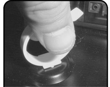
**6** Install two fiber management clips in front of enclosure by inserting into appropriate holes and turning 45 degrees to lock into place (clip opening should face forward).
